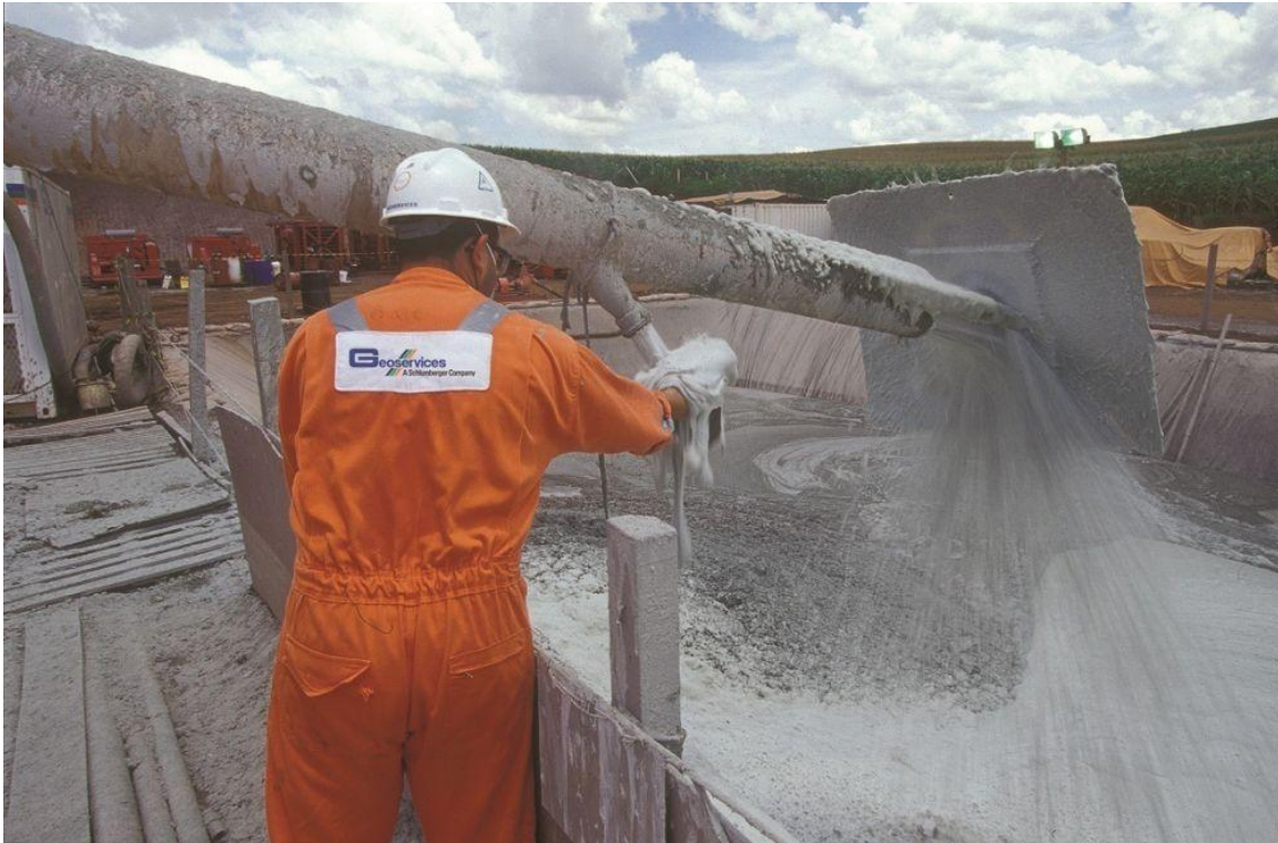
Fig 2 :Mud log in process, a common way to study the rock types when drilling oil wells.
